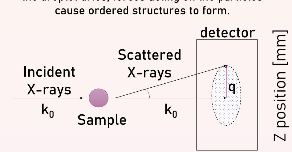
SAXS measurements are taken during the assembly process at various droplet heights (0.1 mm steps). 2D SAXS patterns confirm the shrinking of the droplet in the z-direction due to evaporation and when particle ordering appears.
